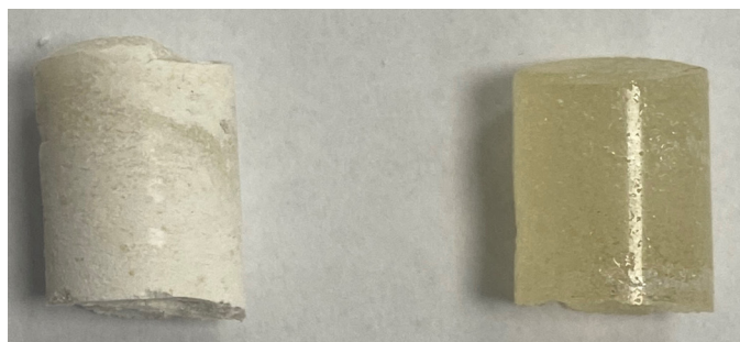
Figure 1 Opaque (left – EFA-PVAL 1-1) and transparent (right – EFA-PVAL 1-5) extrudates obtained in the experiments.
